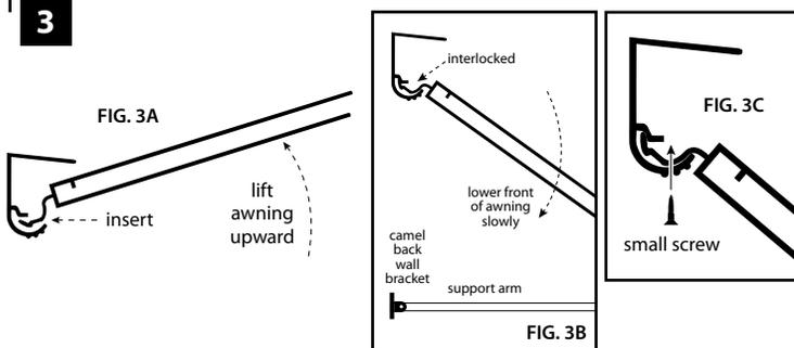
Lift the front of the awning upward and insert the Top Trim into the Mounting Bar (FIG. 3A). Lower the front of the awning slowly and allow Support Arms to rest on the house (FIG. 3B); be sure the two parts are completely interlocked. Align holes and secure Top Trim to Mounting Bar with small screws from bottom side (FIG. 3C).
